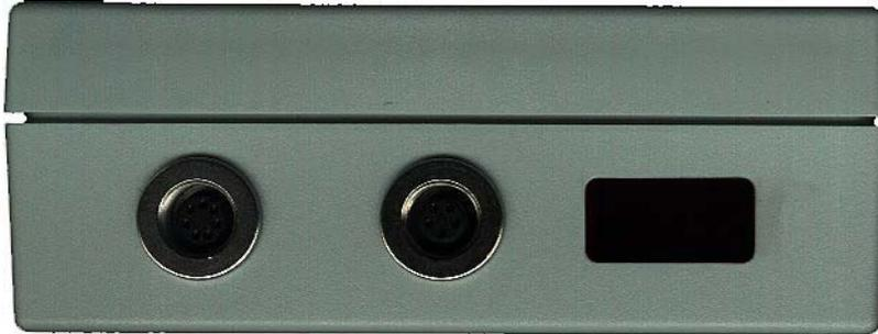
Plug the sensor cable plug into the connection at the measuring device (middle connection – 5 pin).
